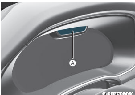
[A] : Interior view camera
