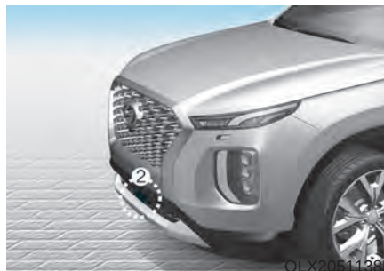
[1]: Front view camera, [2]: Front radar
