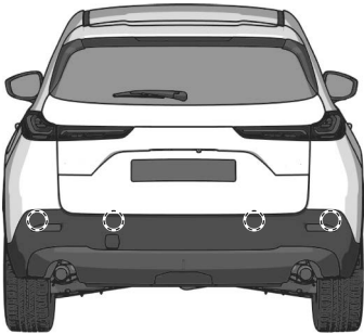
Detection ranges of ultrasonic sensors Vehicles with 360° View Monitor
