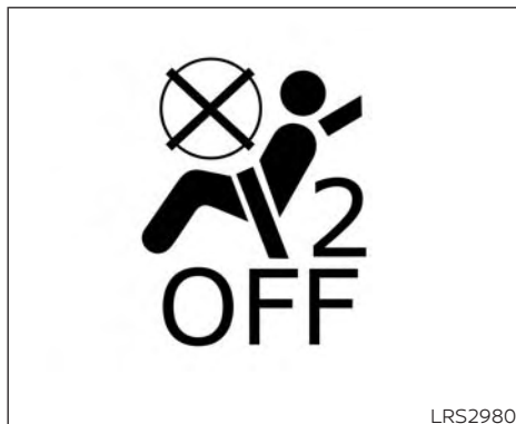
Front passenger air bag and status light
